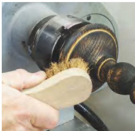
▲ Pic.32 The use of a liming or soft brass brush will remove all the leftover carbon deposits. I have two of these brushes so I don't mind one getting contaminated with black
